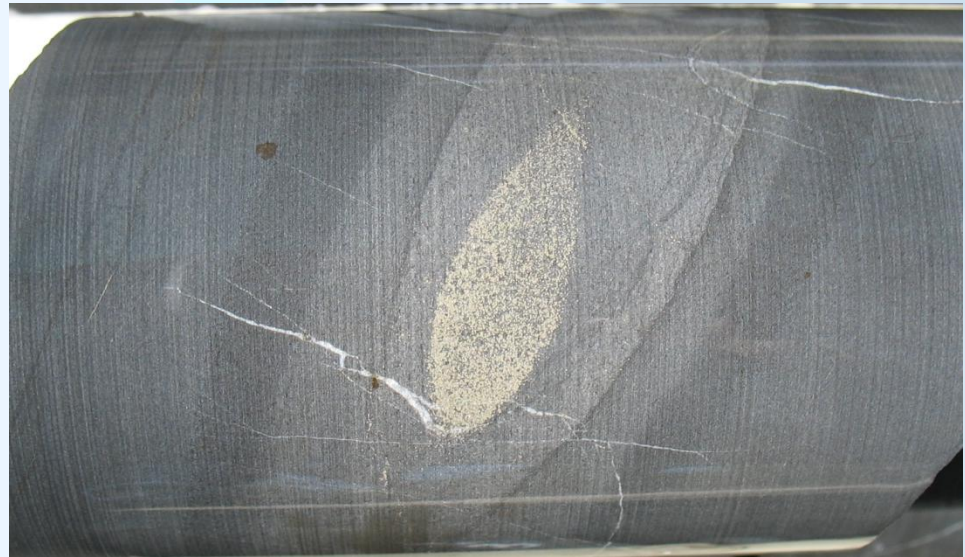
Carbonate concretion with sphalerite in centre
